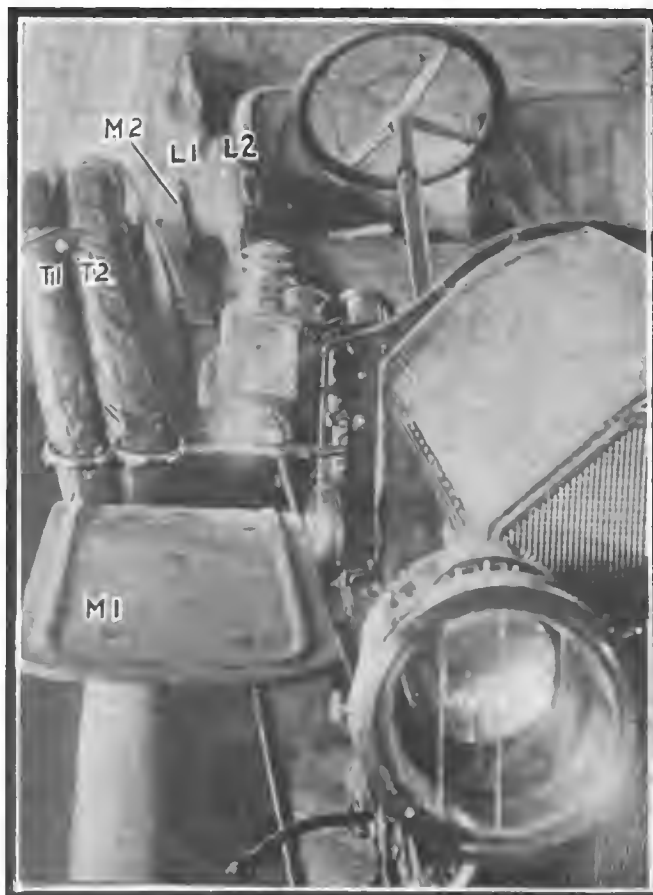
Fig. 1—Method of carrying tires on car with offset levers. This may cause accidents owing to the layover
